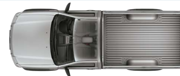
Load box 2280 x 1456 mm. 1235 kg maximum gross payload (1190 kg on 4x2). Double-skinned steel load box with galvanised outer panels and floor. Tie-down rails and rope hooks. 2-position drop-down tailgate. Cab protection frame with ladder stops.
