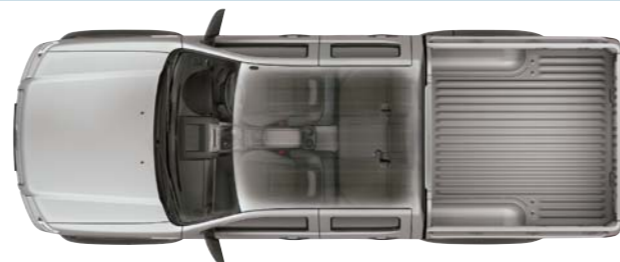
Load box 1530 x 1456 mm. 1175 kg maximum gross payload. 4-door cab style. Double-skinned steel load box with galvanised outer panels and floor. 2-position drop-down tailgate. Cab protection frame with ladder stops. Tie hooks.
